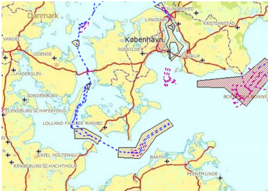
Figure 2 Showing trade fairways (dotted lines) and HELCOM Accident Risk Areas (blocked areas) around Lolland-Falster, excluding ferry lines. Source: EfficienSea ( http://maps.efficientsea.org )
